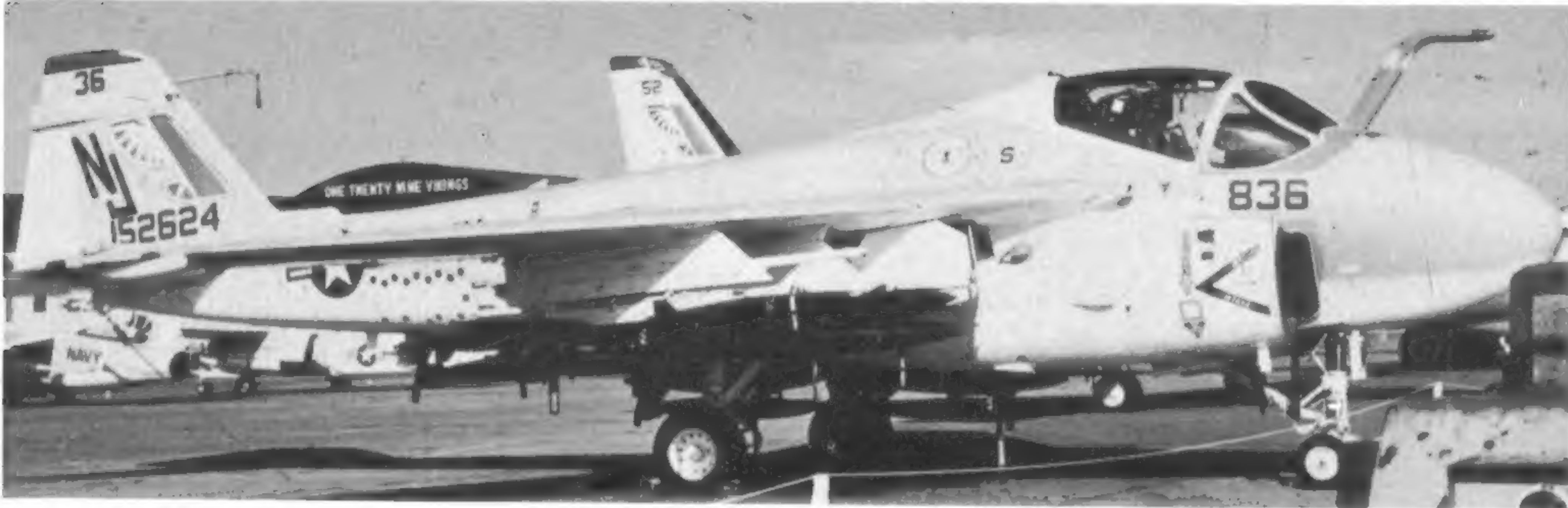
Golden Intruders, VA-128, are flying this A-6A which still has original fuselage speed brakes panels; the brakes no longer operate as is evidenced by paint that remains unburned. (Photo: Bob Labuoy)
