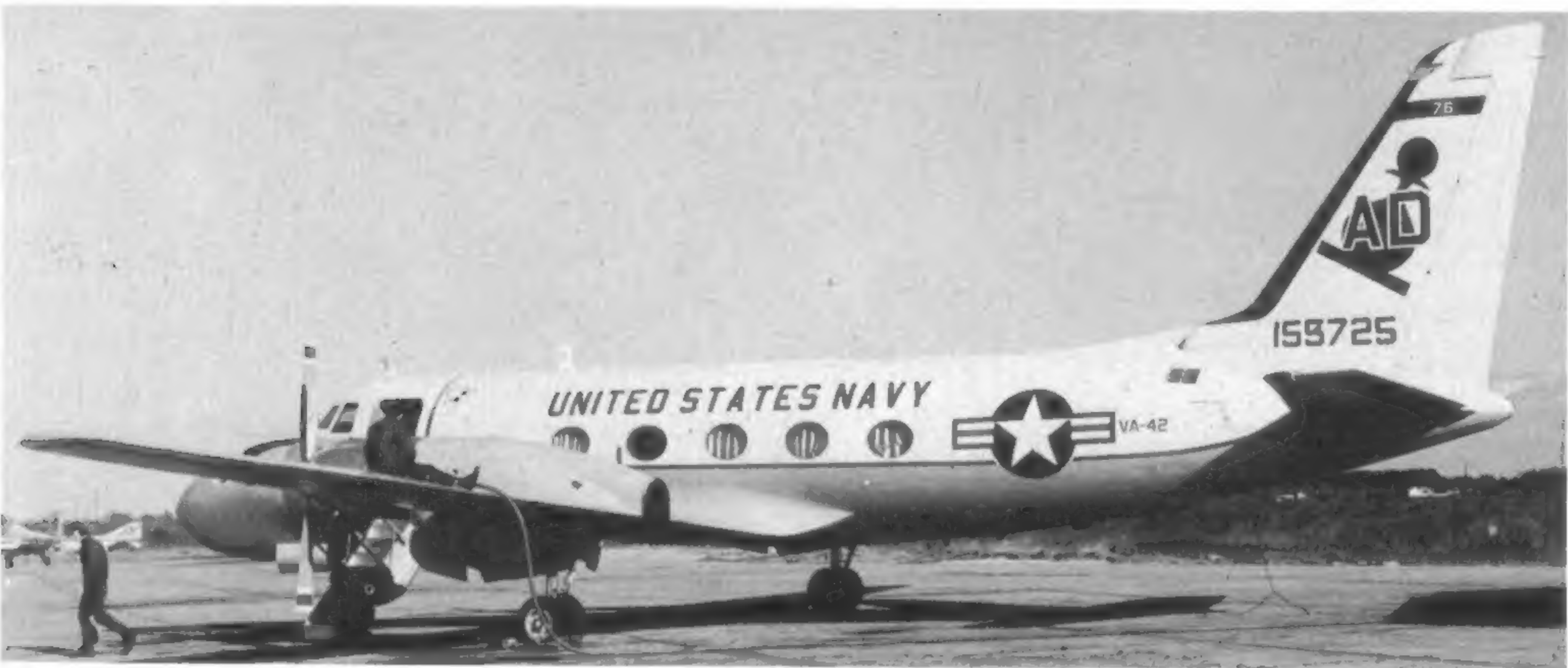
Grumman TC-4C trainer accommodates one A-6 pilot trainee, four B/N trainees and two instructors. Aircraft is equipped with simulated A-6 cockpit, complete attack-nav system and four B/N consoles. Shown is one of VA-42's TC-4Cs. VA-128 and VMAT(AW)-202 also use it. Nine were built; BuNos. 155722 to 155730. (Photo: Author)
