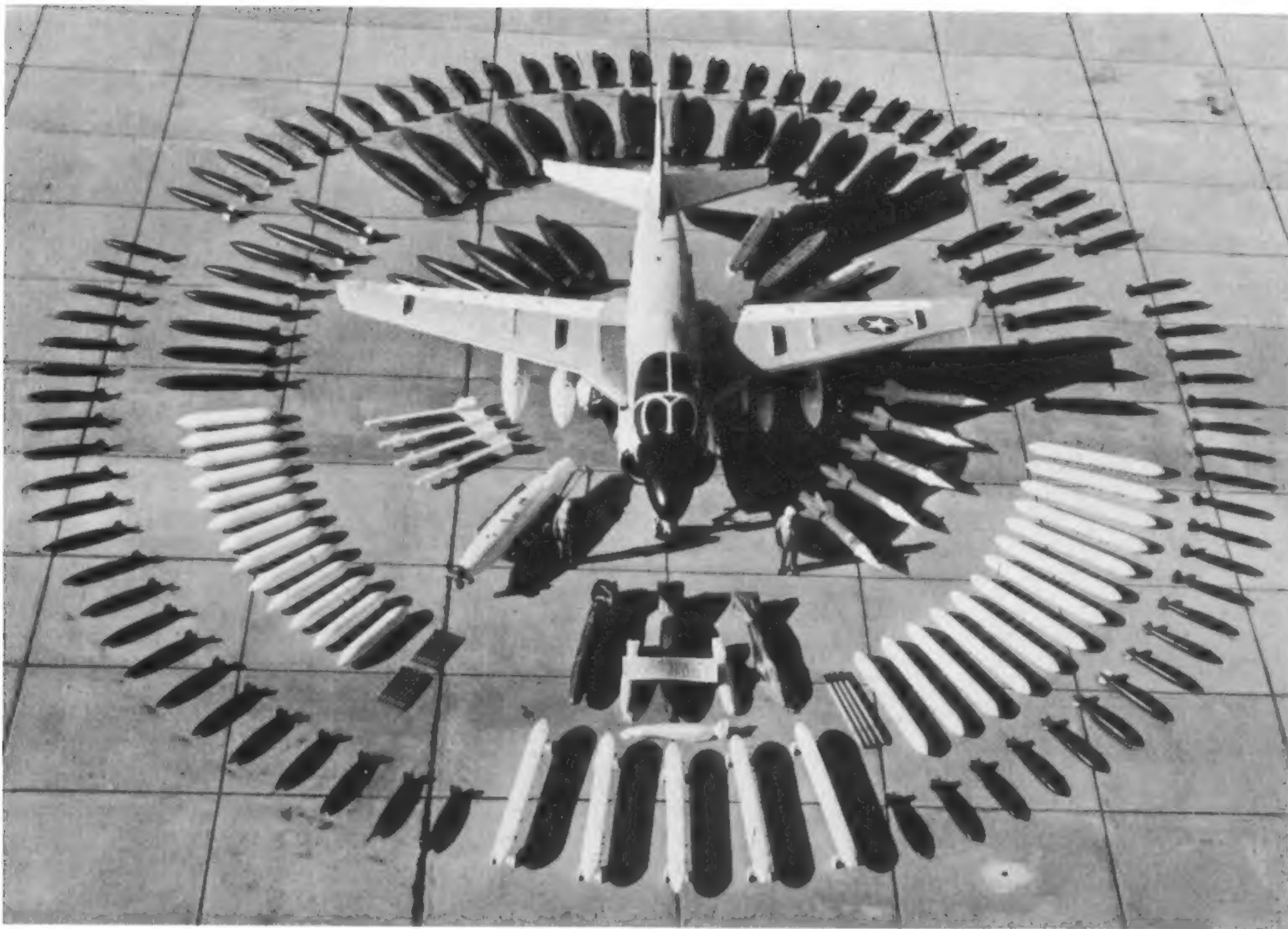
Variety of stores. In outer ring are 500-lb. Mk. 82 (behind) aircraft and 250-lb. Mk. 81 (left and right) general purpose (GP) bombs, with Grumman universal multiple bomb racks in foreground. Second ring includes Mk. 79 fire bombs (behind aircraft), 1000-lb. Mk. 83 GP bombs (left and right), LAU-10/A rocket launchers and 4 of the 5-in. Zuni rockets which they fire (right foreground), AERO 7D rocket launchers and 19 2.75-in. FEAR Mighty Mouse projectiles (left foreground) and some special weapons in front. Immediately behind A-6, left, are 2,000-lb. Mk. 84 GP bombs and, right, AERO 8A practice bomb containers. In front of wings, left, are 4 Sidewinder IC missiles and a 300-gal. refuelling store. In front of wings, right, are 5 Bullpup missiles and 5 300-gal. tanks are on aircraft. (Photo: Grumman 62213)
