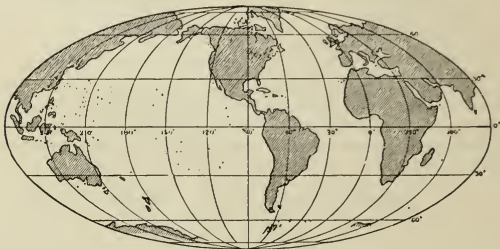
FIG. 12.—The Mollweide equal-area projection of the sphere.
