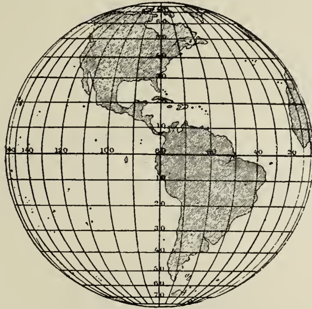
FIG. 33.—Orthographic projection of the Western Hemisphere.
