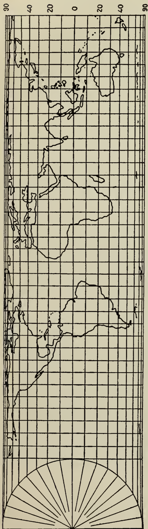
FIG. 16.—Cylindrical equal-area projection.
