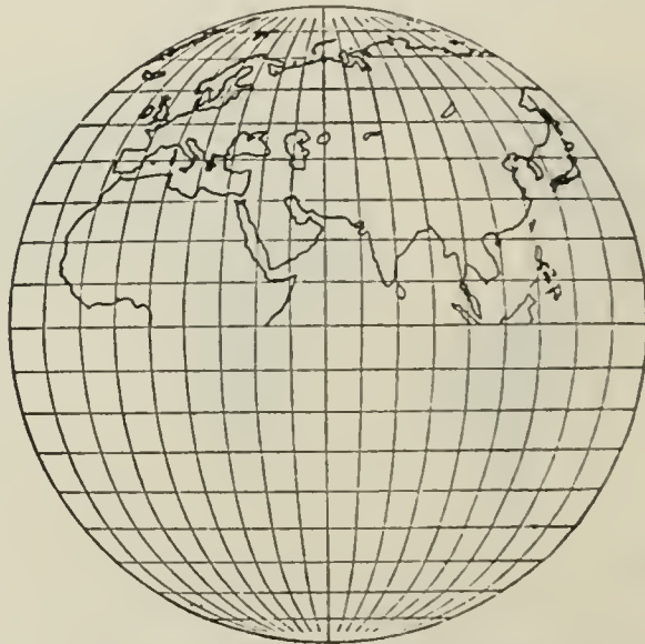
FIG. 72.—The Mollweide homolographic projection of a hemisphere.
